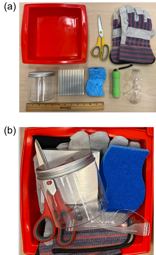
Figure 1. (a): A photo of an unassembled kit is shown: black construction paper, sponge, heat sink, gloves, scissors, eye protection, and plastic jar with lid. (b): A photo of an unassembled kit in storage is shown. All components fit in the silicone baking pan for organized storage of each kit as an individual unit.
